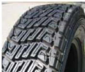
**RB3** – This is an all purpose forest tyre, capable of optimum performance on a variety of terrain, it is produced in aspect ratios from 55-70 series to optimize gearing
